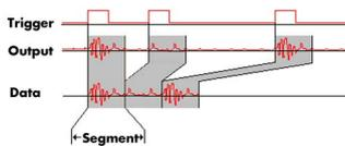
The Multiple Replay mode allows the fast output generation on several trigger events without restarting the hardware. With this option very fast repetition rates can be
