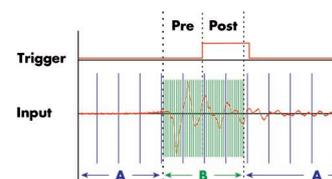
The ABA mode combines slow continuous data recording with fast acquisition on trigger events. The ABA mode works like a slow data logger combined with a fast digitizer. The exact
