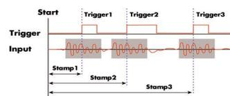
The timestamp function writes the time positions of the trigger events in an extra memory. The timestamps are relative to the start of recording, a defined zero time, externally synchronized to a radio clock, an IRIG-B or a GPS receiver.
